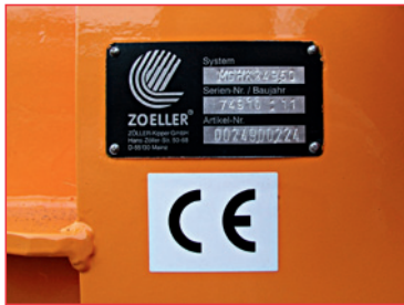
✓ Manufacturers plate with required information and separate CE Mark
