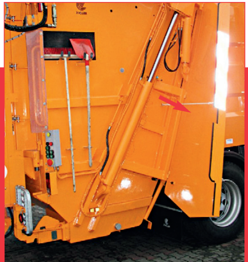
✓ Lockable side cover doors for shear protection
