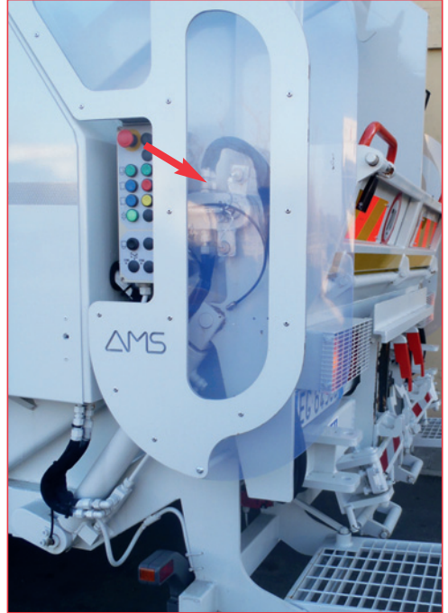
✓ Transparent and flexible guards covering shearing and crushing zones at the lifting device
