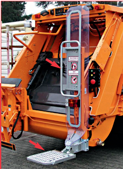
✓ Ergonomic positioning of footboards and handrails in operation position
