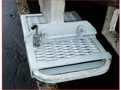
X Footboard – with insufficient dimensions of the fixed part and non controlled extensible part which could induce misuse
