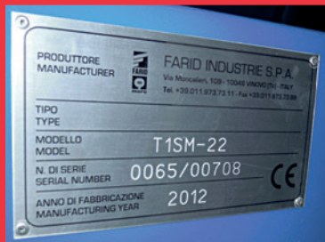
✓ Manufacturers plate with required information including CE Mark
