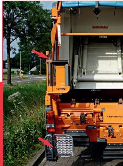
✓ Folded footboards and handrails in transport position
