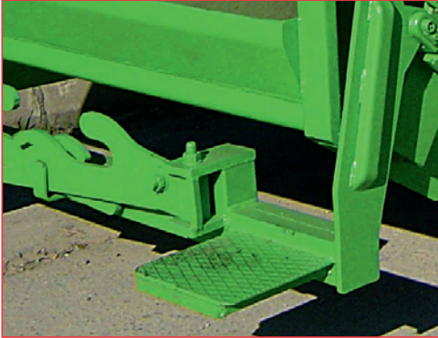
X Footboard – not tiltable, without detection system and without anti-slip surface
